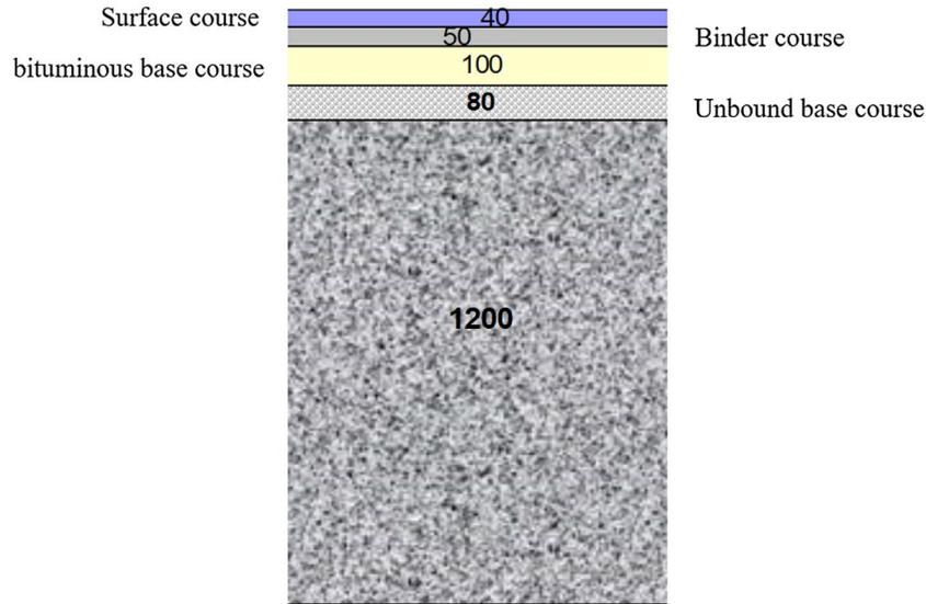
**Figure 1.** Test structure with layer thicknesses in mm.
