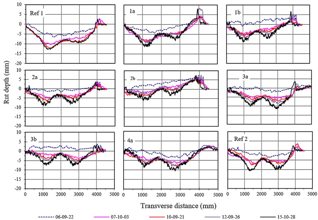
Figure 13. Transverse profiles of the test sections developed over time.
