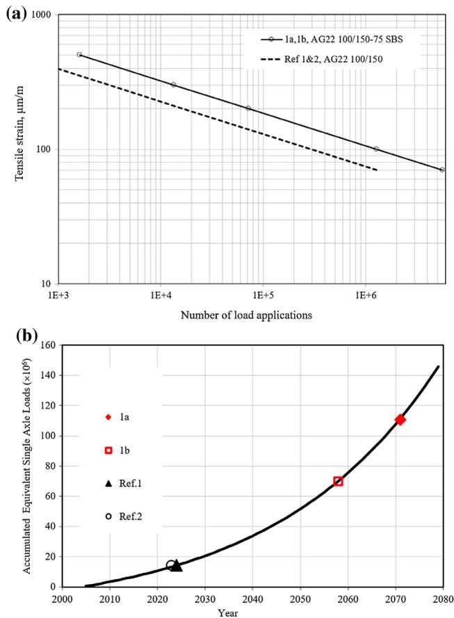
**Figure 17.** Laboratory-determined fatigue life relationships (a) and service lives of pavement structures based on estimated strains from FWD deflection measurements at  $10^\circ\text{C}$  (b).
