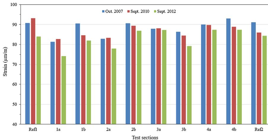
Figure 12. Estimated horizontal strain at the bottom of the bituminous layers adjusted to 10 °C.
