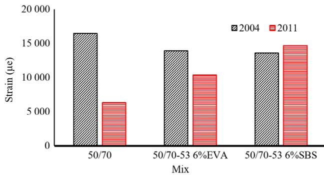
Figure 8. RLCT creep strain of the binder mixes from 2004 and 2011.
