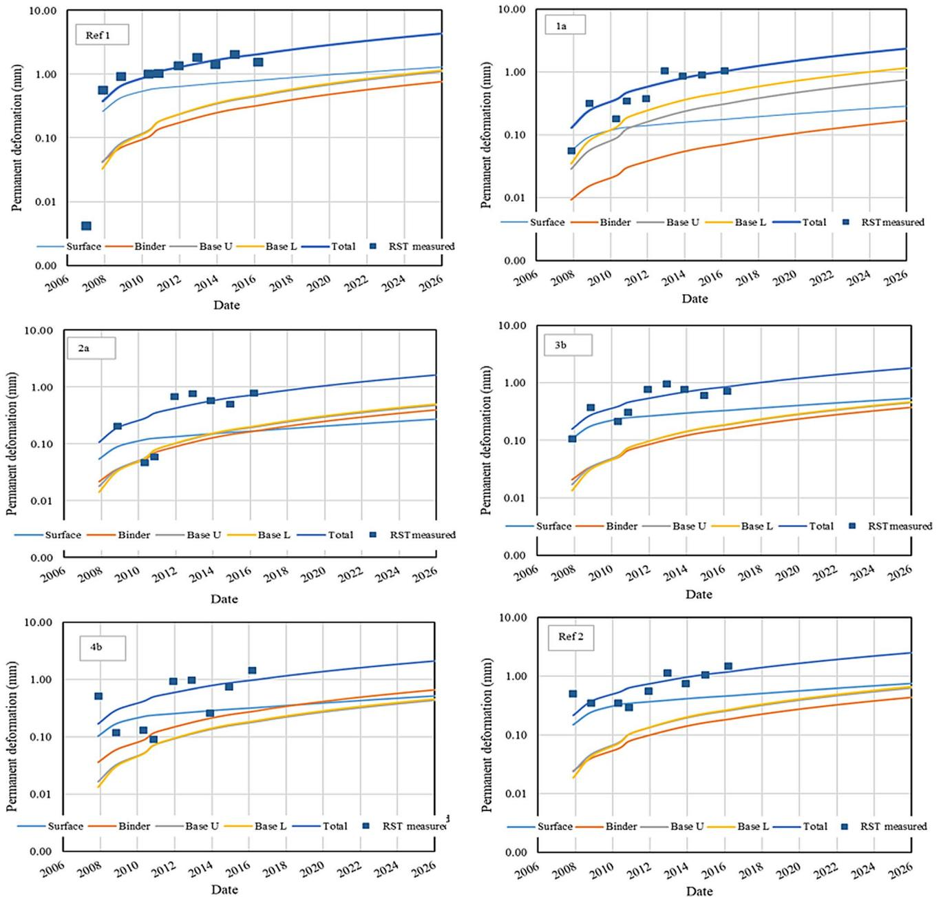
Figure 20. Measured and modelled permanent deformation of the pavement structures.
