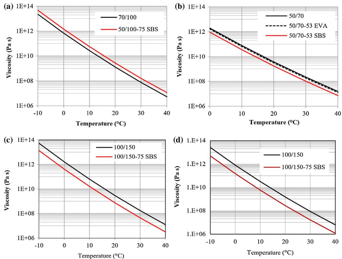
Figure 6. Complex viscosity at peak phase angle; (a) surfacing (SMA 16), (b) binder course (ABb 22) and (c) and (d) upper and lower base courses (AG 22), respectively.
