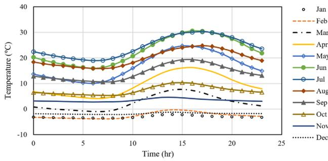
Figure 19. Monthly and hourly temperature variation at 2 cm below the surface.
