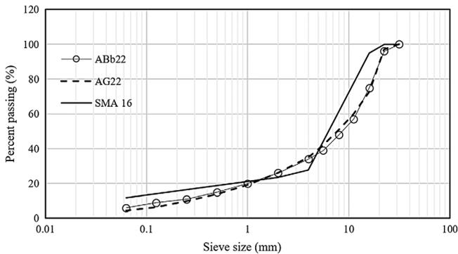
**Figure 2.** Grain size distribution of the surface, binder and base course mixes.
