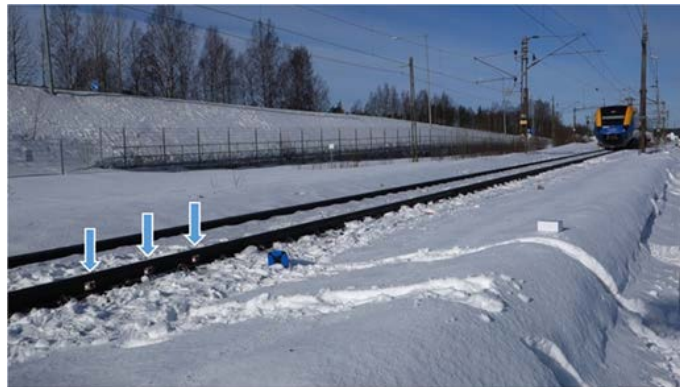
Figure 1: Test of three MEMS wake-up circuits of the same model (Lindqvist, 2017).
